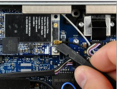
Use the flat end of a spudger to pry both antenna connectors up off the AirPort Extreme card.
