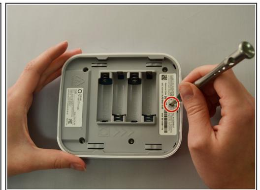
**⚠** Make sure the batteries are removed before attempting disassembly.
