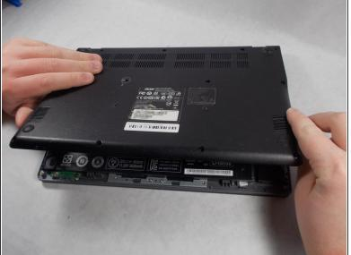
Pry the back panel open with the plastic opening tool.
