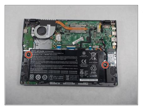
Remove the two 6.0mm screws securing the battery with your Phillips #1 screwdriver.
