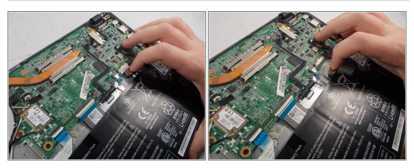
Carefully pull out the battery wire connected to the battery port.
