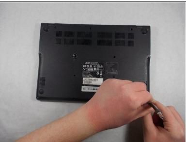
Remove the thirteen 6.0mm screws on the back panel using your Phillips #1 screwdriver.
