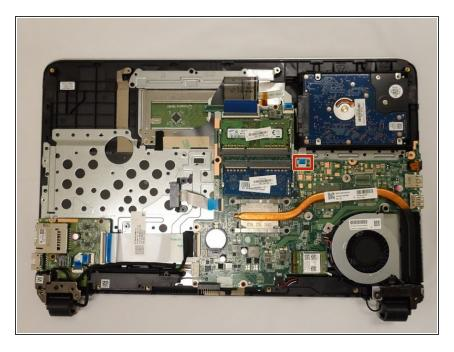
Locate the ribbon cable connecting the hard drive to the motherboard.
