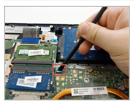
On the motherboard, lift the white tab up to release the ribbon cable.
