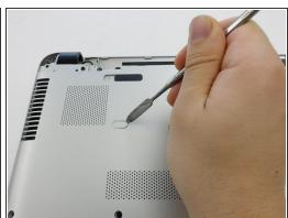
Remove the two plastic tabs with a metal spudger.
