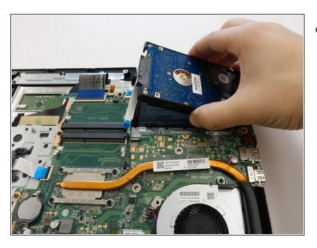
Pull the hard drive out of the enclosure.
