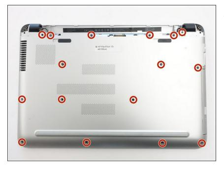
Remove the sixteen 8mm screws that hold the bottom cover with a Phillips #1 screwdriver.
