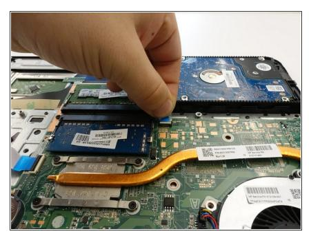
Pull the blue tab up and out from the motherboard to disconnect the ribbon cable.
