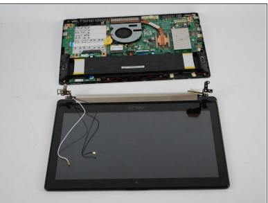
Remove the bottom of the laptop from the screen.
