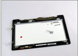
• Use a sharp object to remove tape from the back of the screen.
