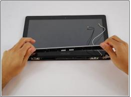
Remove the hinge cover by gently pulling to the right then upwards.
