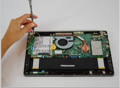
Using a Phillips #1 Screwdriver unscrew the four 4 mm screws holding the screen holder onto the motherboard.
