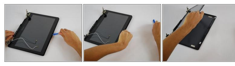
Push screen downwards then pull top of screen upwards and remove the screen.
