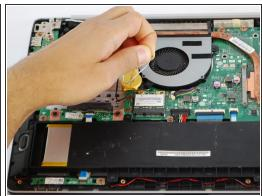
Remove the two cables connecting to the wifi card.
