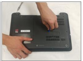
Using a plastic opening tool, pry the back panel from the computer, going all the way around it.
