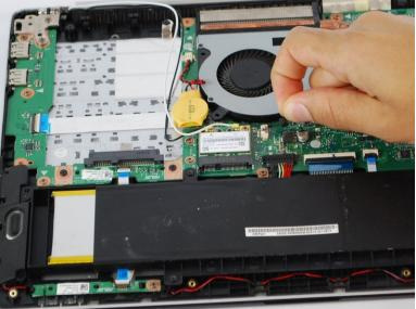
Remove the wire connecting the fan to the motherboard.
