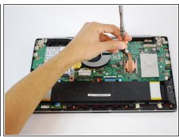
Using a Phillips #1 Screwdriver remove the three 3 mm black screws and four 2 mm copper screws holding the fan and heat sink in place.
