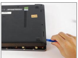
• Use a plastic opening tool to gently pry the bottom of the laptop up. Slowly slide it along the edges, twisting it every so often to pop the bottom of the laptop out of the clips holding it in place.
