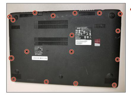
• Use a Phillips #0 screwdriver to remove seventeen 7mm screws from the lower case.
