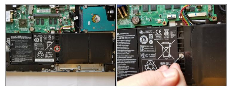
• Remove the PH #0 screw from the center of the battery.
