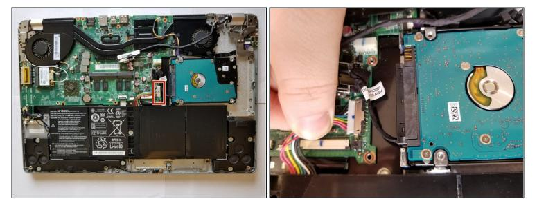
• Pull the battery connector away from the hard drive to disconnect it from its socket.
