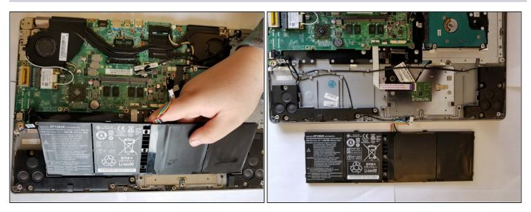
• Lift up the battery to remove it.
