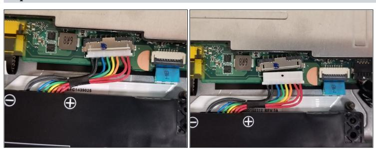
• Pull the rainbow cord out of the motherboard using the tabs on the sides.
