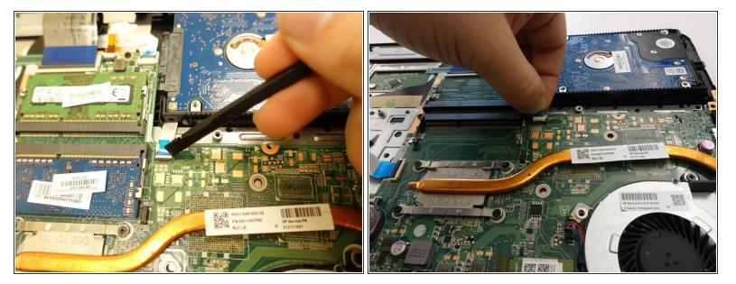
Unlock and remove the cable that connects to the hard drive.
