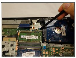
Unlock and remove the cables connected to the keyboard.
