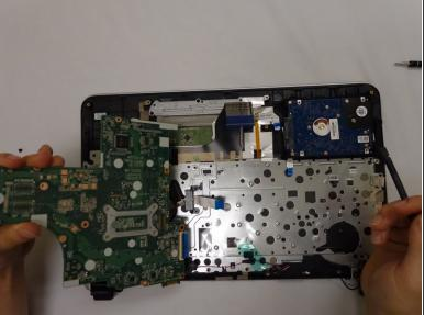
• Lift the motherboard up and flip it around to reveal the cable connected on the underside.
