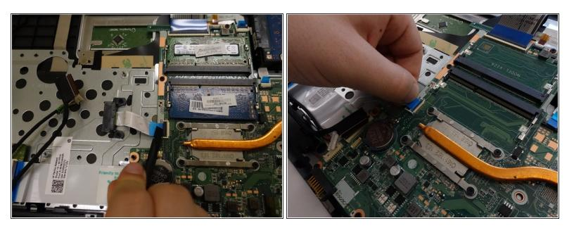
Unlock and remove the cable connected to the optical drive.
