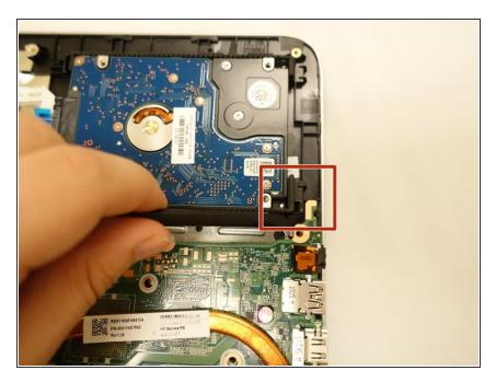
Release motherboard from the clip at the base of the hard drive.
