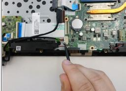
Unlock and disconnect cables attached to the motherboard that connect to the display.
