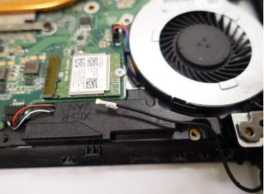
Disconnect the wire connected to the Wifi card.
