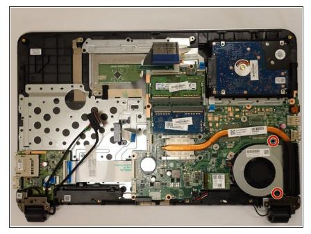
Remove the 4mm screws holding the motherboard in place with a Phillips #1 screwdriver.
