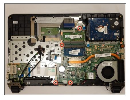
Remove the 4mm screws holding the motherboard in place with a Phillips #1 screwdriver.
