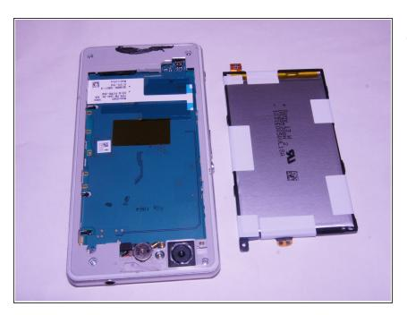
Remove the battery from the device
