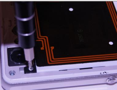
Remove the single 1 x 3.0 mm screw holding the battery in using the JIS #00 screwdriver.
