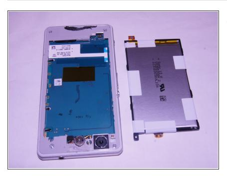
Remove the battery from the device
