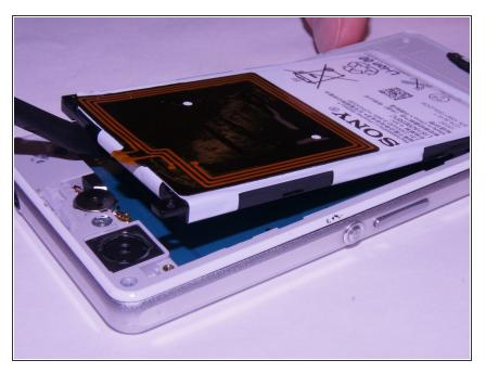
Pry the battery up from the ends using the plastic spudger until the battery pops out of the enclosure.
